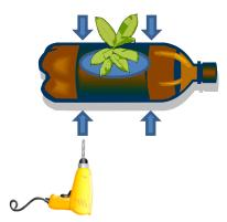
Keep the cap on when you're drilling and be VERY careful when you're cutting out the hole with box cutters or scissors.
